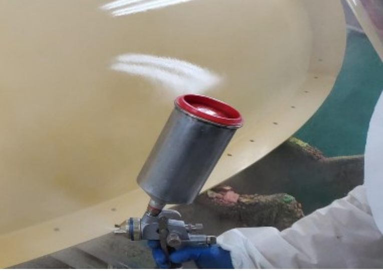
Figure 72: Spray in Controlled Area with Full PPE
