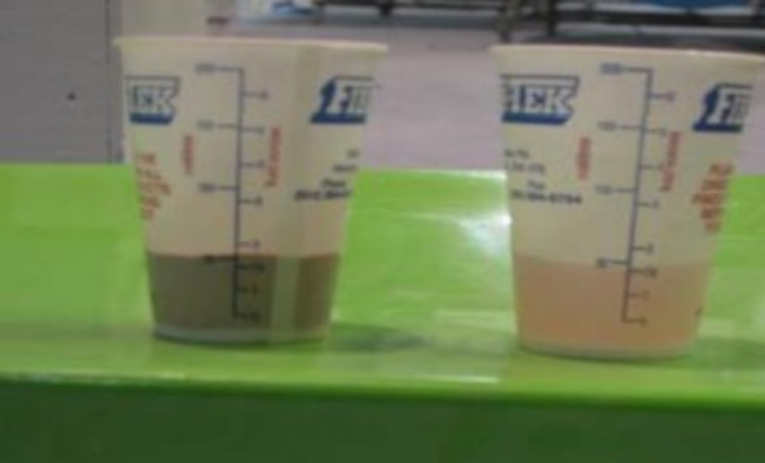
Figure 48: Pour Equal Gelcoat and Pro Patch Amounts
