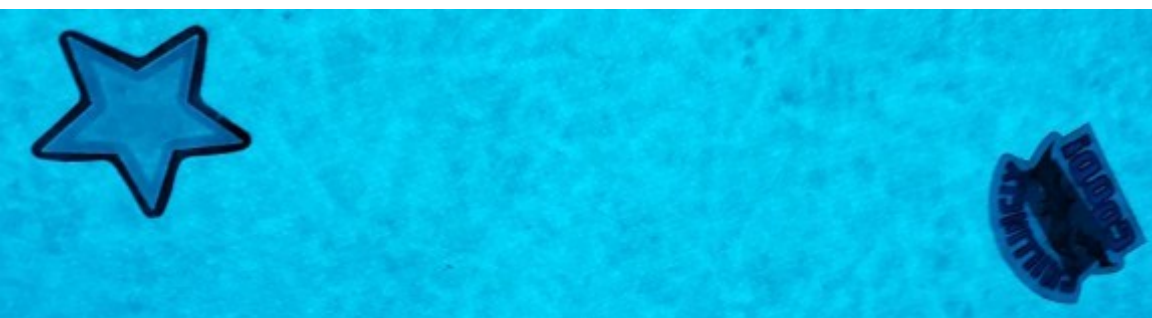
Figure 4: Stickers and Adhesive Glue on FRP
