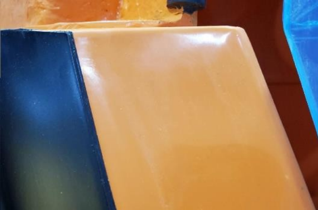
Figure 67: Buffed Small Putty Repair
