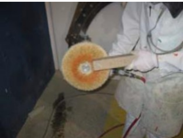
Figure 65: Apply Buffing Compound to Pad
