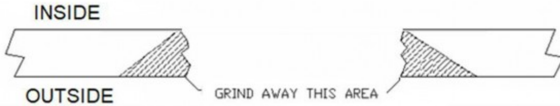
Figure 28: Grind Away Repair Area
