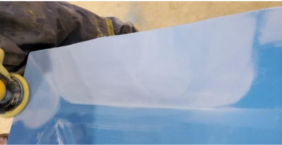
Figure 55: Sand with 400 to 600 grit Sandpaper
