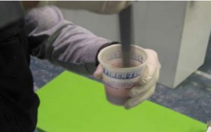
Figure 49: Mix Gelcoat and Pro Patch
