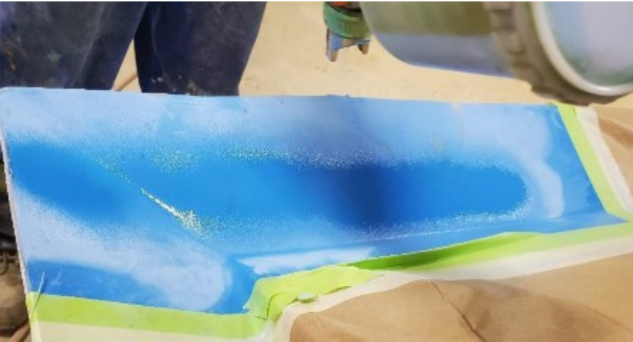
Figure 53: Spray on an Even Coat
