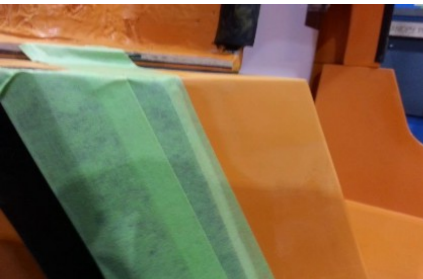
Figure 44: Sanded Gelcoat Putty Repair
