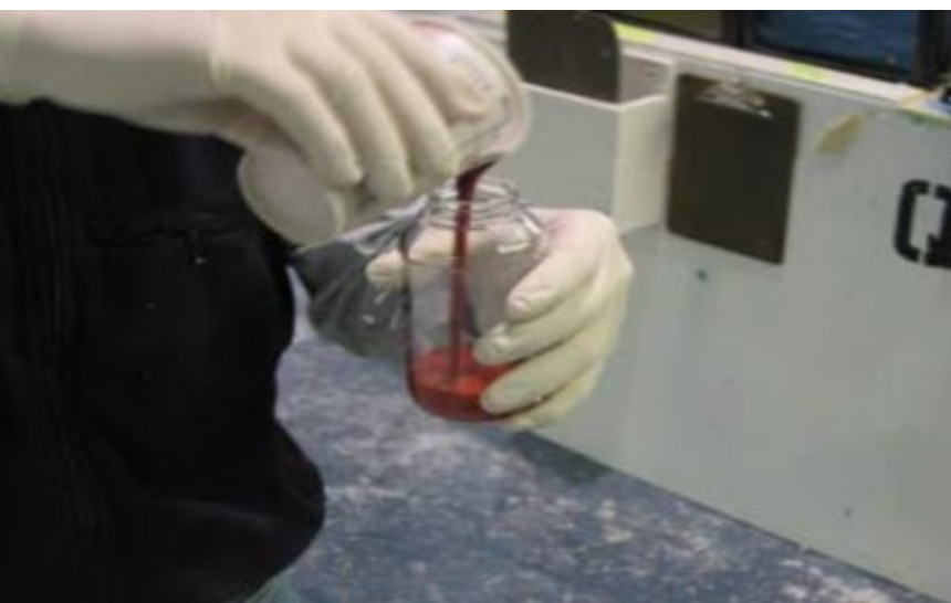
Figure 51: Pour Mixture into Spray Paint Jar
