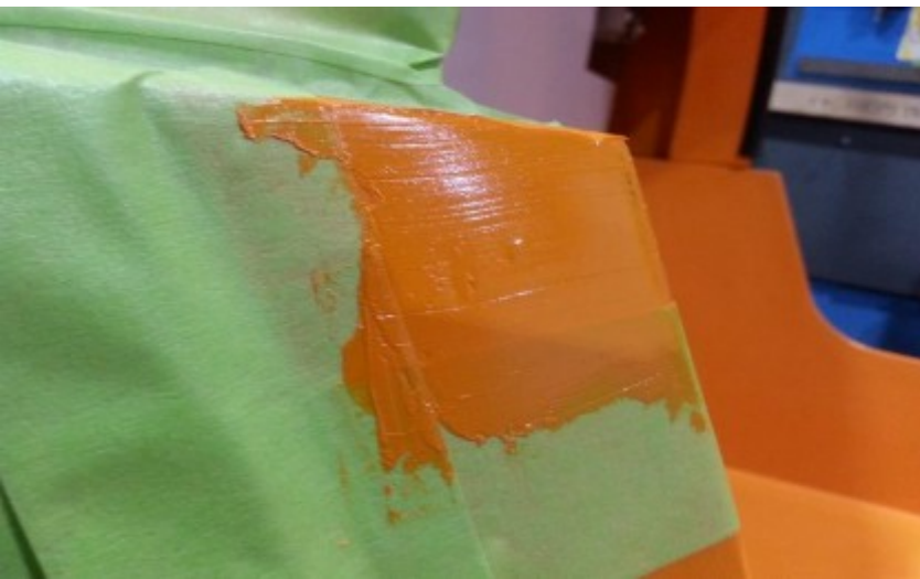
Figure 43: Applying Gelcoat Putty
