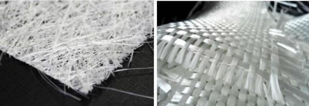
Figure 33: Chopped Strand Mat and Woven Roving
