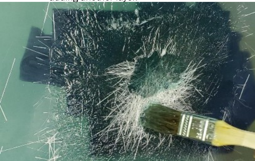
Figure 38: Soak Fiberglass with Paint Brush
