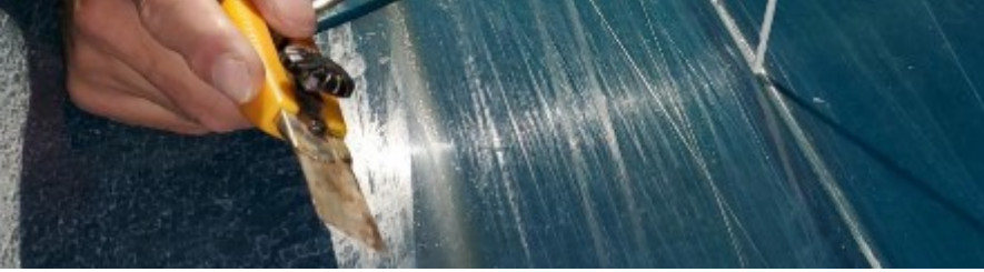
Figure 7: Removing Old Filler
