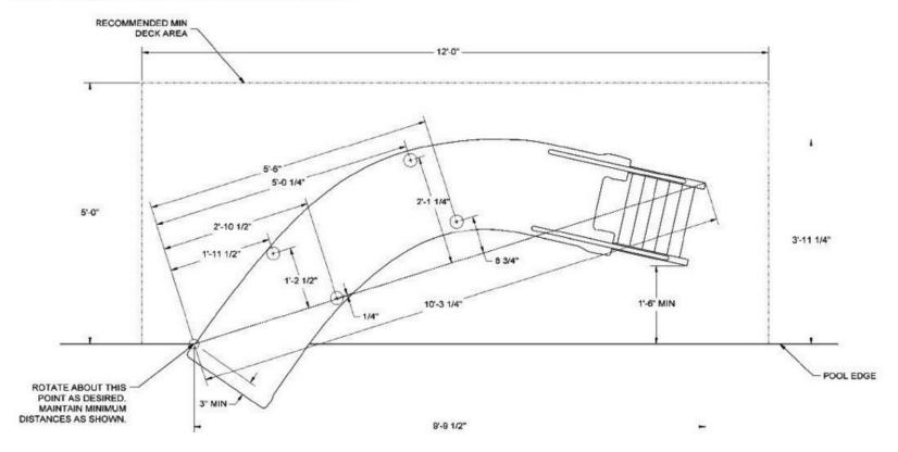
**NOTE:** FINAL POSITION MUST ENSURE THAT ALL WATER FALLING OFF SLIDE LANDS IN POOL. DIMENSIONS MAY VARY FROM SLIDE TO SLIDE. IT IS RECOMMENDED THAT THE FULLY ASSEMBLED SLIDE BE USED AS A TEMPLATE FOR INSTALLATION.
