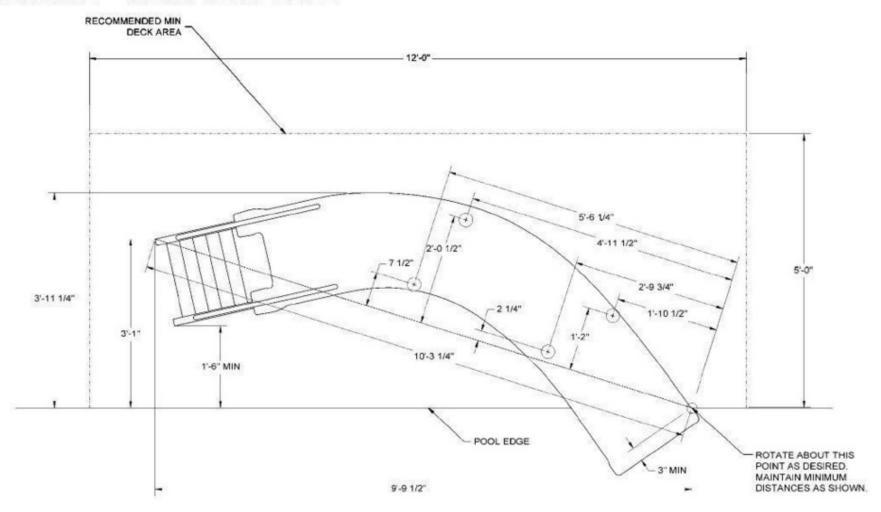
**NOTE:** FINAL POSITION MUST ENSURE THAT ALL WATER FALLING OFF SLIDE LANDS IN POOL. DIMENSIONS MAY VARY FROM SLIDE TO SLIDE. IT IS RECOMMENDED THAT THE FULLY ASSEMBLED SLIDE BE USED AS A TEMPLATE FOR INSTALLATION.
